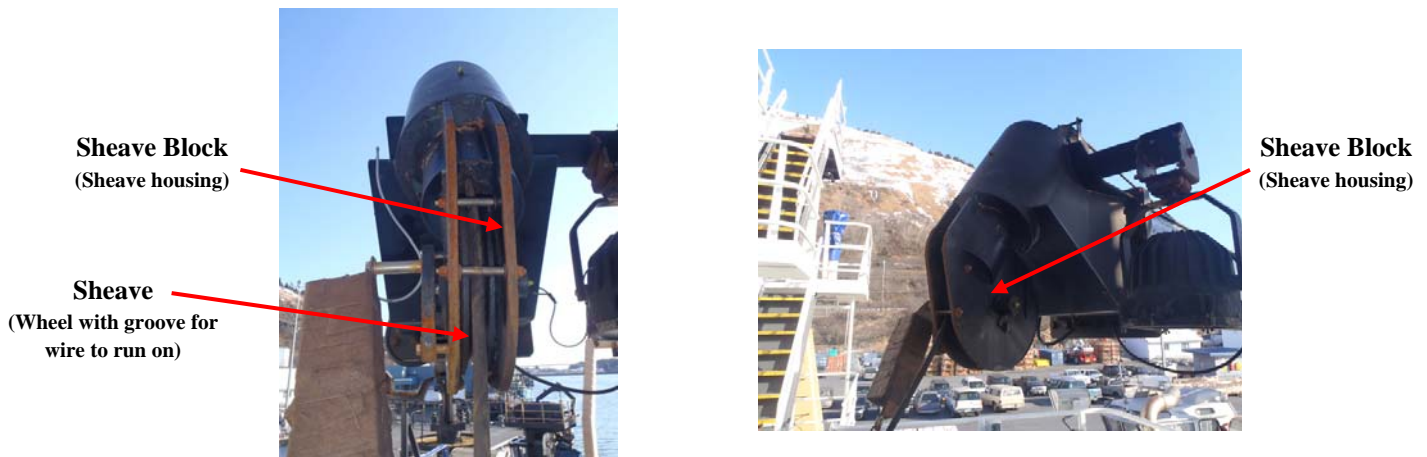
Figure 4. Starboard Crane sheave and sheave block
