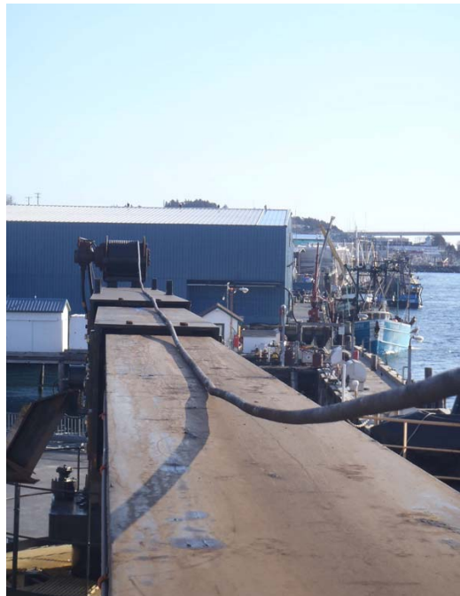
Figure 6. Deformed existing wire rope on Starboard crane
