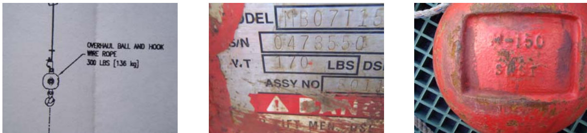
Figure 3. Overhaul (headache) ball weights (left - crane manual diagram; center - port crane; right - starboard crane)
