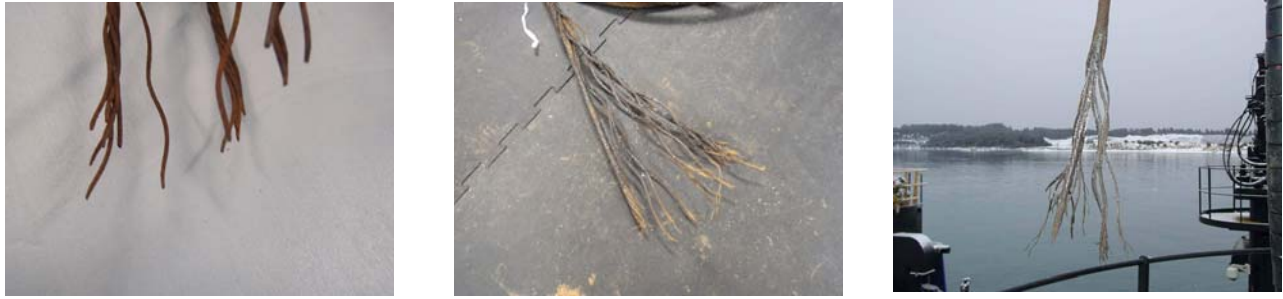
Figure 6. Deformed existing wire rope on Starboard crane
